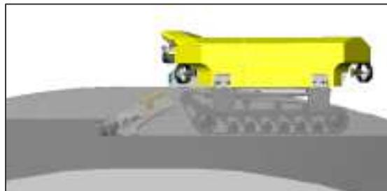
**Figure 3-3: ROV with drum cutter**
