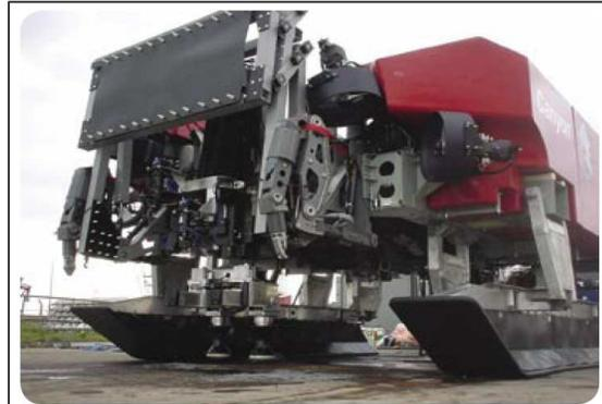
*Nautilus has investigated the use of proven subsea technology for mining the SMS deposits. This 900HP ROV oil/gas pipelay trenching machine is as powerful as a D11 bulldozer.*
